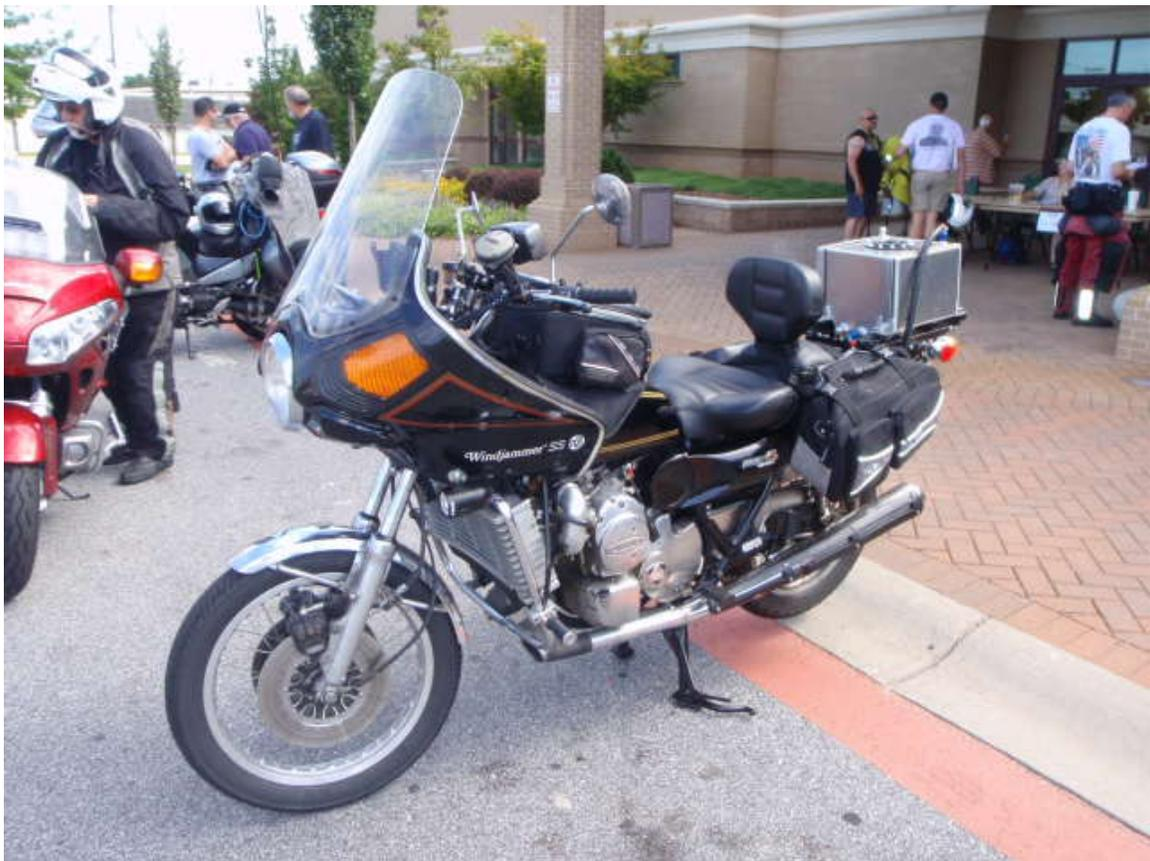
**1976 Suzuki RE-5 Rotary Engine-Powered Motorcycle**
